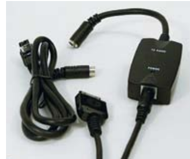
IPOD ADAPTORS. These connect an iPod to a stereo and not only play music from the portable player, but also charge it and allow it to be controlled from the stereo or a remote. The adaptor shown here is for a Clarion stereo.
